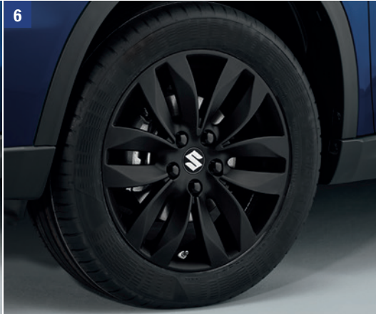
6 | Alloy Wheel "MISTI" WVTA Matte Black painted, 6.5 J x 17" suitable for 215/55 R17 tires, including centre cap with S logo. Part No. 43210-61MQ1-Y12
