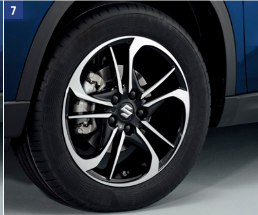
7 | Alloy Wheel "MOJAVE" WVTA Black Polished, 6.5 J x 17" suitable for 215/55 R17 tires, including centre cap with S logo. Part No. 43210-54PU1-0SP A D
