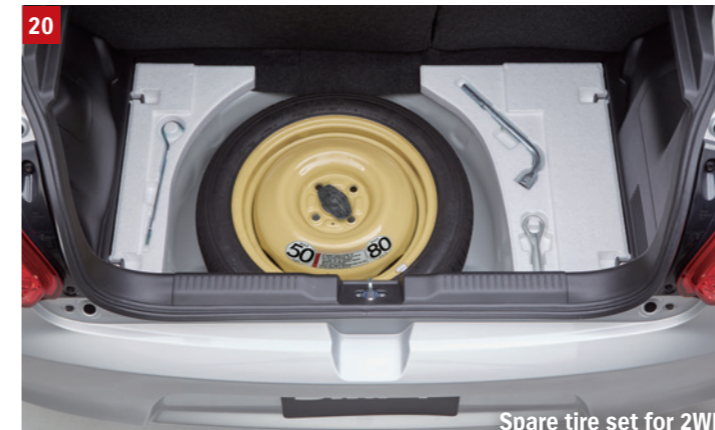
20 | SPARE TIRE KIT for 2WD 1,2 Includes spare tire kit, fixation kit, jack and jack bracket kit. Part No. 990E0-STSW2-001
