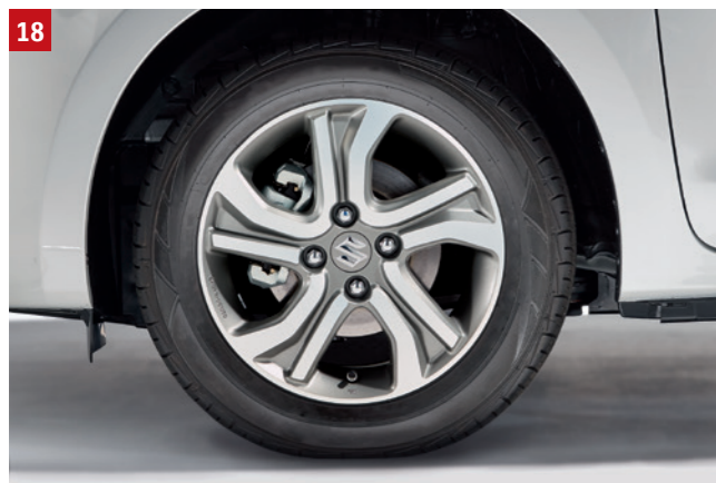
18 | ALLOY WHEEL "COSMIC" Metal gray matte polished, 5x15" alloy wheel for 175/65R15 tires, centre cap with Suzuki logo. ECE R124 and JWL approval. Part No. 43210-52RS0-000
